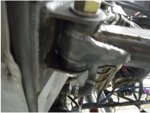
Bottom view of installed wrap on lower trailing arm
