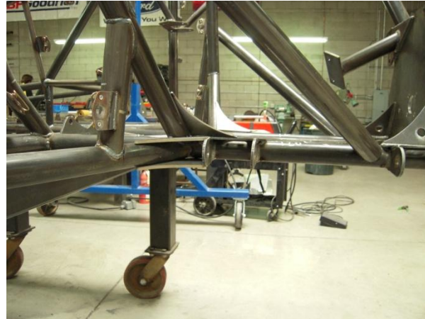
Side view of the plates and tube installation.
