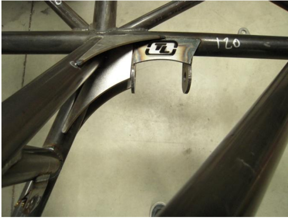
Top view of the plates installed in the chassis.
