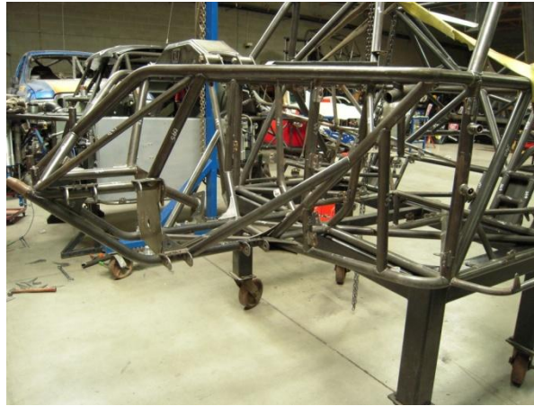
Side view of the truck chassis with the tubes and plates installed. The tubes run from just behind the lower front arm mount up to the tube in the firewall. You will have to split the front firewall aluminum panel into two parts to install it after the tube is in place.
